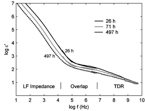
FIG. 3. Wide-range frequency dependence of the real permittivity during long-time OPC cure, using the combined TDR and low-frequency measurement ( $w/c=0.4$ ,  $23^\circ\text{C}$ ).
