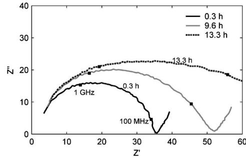
FIG. 5. Complex impedance during an early OPC cure, corresponding to the real permittivity in Fig. 2 and the dielectric conductivity in Fig. 4 ( $w/c=0.4$ ,  $23^\circ\text{C}$ ).
