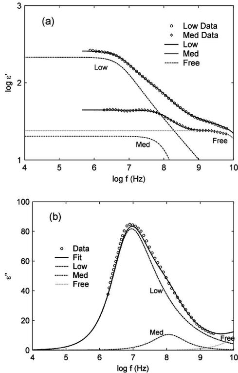
FIG. 7. Subtracted model fit for OPC at 15-h cure, showing the low- and medium-relaxation components for the real permittivity, and the combined low- and medium-relaxation fit for the imaginary permittivity ( $w/c=0.4$ ,  $23^\circ\text{C}$ ).
