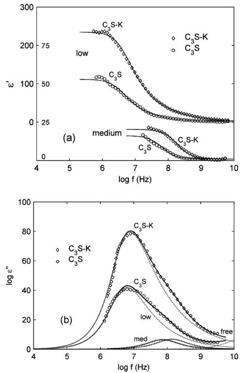
FIG. 11. Effect of ionic strength on the  $C_3S$  paste at 19-h cure, showing the subtracted low- and medium-relaxation components for real permittivity and the combined low- and medium-relaxation fit for imaginary permittivity for both samples ( $w/c=0.4$ ,  $23^\circ C$ ).
