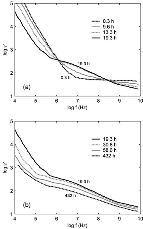
FIG. 2. Frequency dependence of the real permittivity during OPC cure ( $w/c=0.4$ ,  $23^\circ\text{C}$ ).
