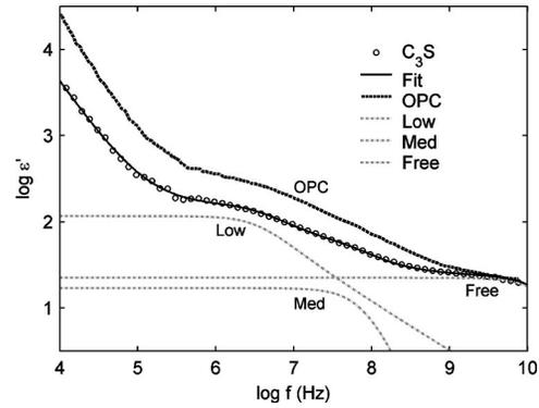
FIG. 9. Representative model fit for the  $\text{C}_3\text{S}$  paste at 21-h cure, showing the individual model components along with combined fit ( $w/c=0.4$ ,  $23^\circ\text{C}$ ). The OPC model fit at 21 h overlaid for comparison.
