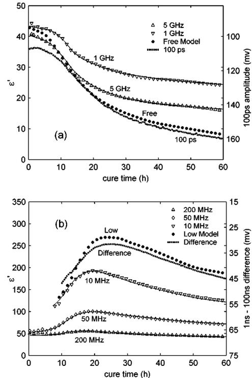
FIG. 12. Constant-frequency permittivities during OPC cure as extracted from Fig. 2. Permittivities at 1 and 5 GHz compared to the free-relaxation model and permittivities at 10, 50, and 200 MHz compared to the low-relaxation model, with model-predicted permittivities overlaid on measured values. The 100-ps transient amplitude and (1–100 ns) difference signal overlaid for comparison ( $w/c=0.4$ ,  $23^\circ\text{C}$ ).
