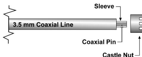
FIG. 1. Schematic of cement sensor.
