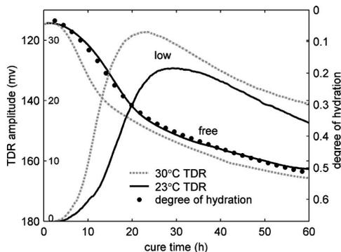
FIG. 14. Evolution of the free- and low-relaxation indicators during OPC cure for the two pastes cured at 23 and  $30^\circ\text{C}$  ( $w/c=0.4$ ). Comparison of the free-relaxation indicator with the degree of hydration as measured by isothermal calorimetry.
