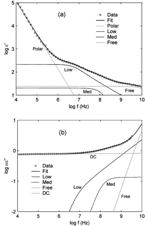
FIG. 6. Representative model fit for OPC at 15-h cure, showing the individual model components along with combined fit. The real permittivity and dielectric conductivity are fit using shared parameters ( $w/c=0.4$ ,  $23^\circ\text{C}$ ).
