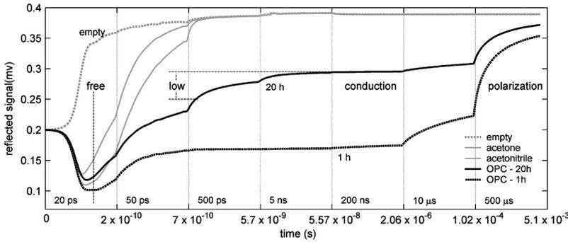
FIG. 13. Direct TDR transient captured on the nonuniform time scale, showing the empty-sensor and reference reflection ( $\epsilon' = 21.1, 37.5$ ) along with the OPC reflection at 1 and 20-h cure. The location of the transient amplitudes identified for both the free- and low-relaxation indicators ( $w/c=0.4, 23^\circ\text{C}$ ).
