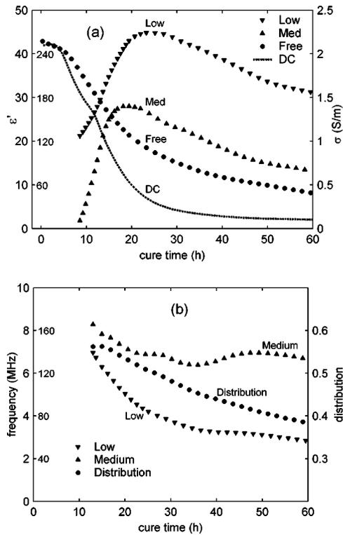
FIG. 8. Evolution of model parameters during OPC cure, showing the relaxation amplitudes, frequencies, and distributions factors as a function of cure time ( $w/c=0.4$ ,  $23^\circ\text{C}$ ).
