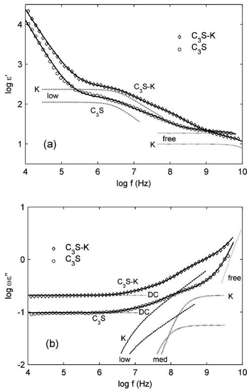
FIG. 10. Effect of ionic strength on the  $C_3S$  paste at 19-h cure, showing the individual model components along with the combined fit for both samples ( $w/c=0.4$ ,  $23^\circ C$ ).
