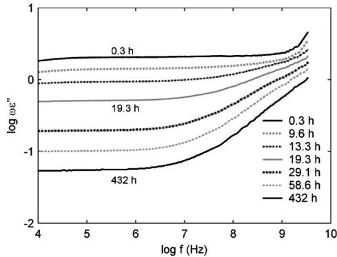
FIG. 4. Frequency dependence of the dielectric conductivity  $\omega\epsilon''$  during OPC cure, corresponding to the real permittivity in Fig. 2 ( $w/c=0.4$ ,  $23^\circ\text{C}$ ).
